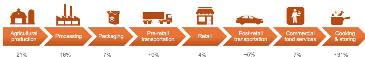
**FIGURE 1. Generic life cycle of food production with the distribution of the estimated 10.8 EJ of energy used annually by the US food system based on data from the early to mid-1990s. Adapted from Heller and Keoleian, 2003. (EJ = 10<sup>18</sup> J).**
